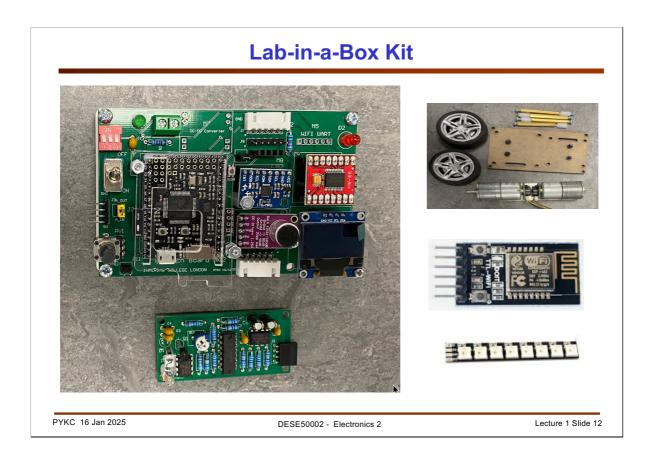
The Lab-in-a-Box Kit for this module consist for two bespoke (i.e. purpose built) boards. The main board is known as the PyBench unit. It consists of the main processor board (Pyboard), motor driver, display, microphone with automatic gain amplifier and an IMU. Unlike last year or Gizmo, you DO NOT need to build any circuits. These are modules are all connected together with a PCB.
